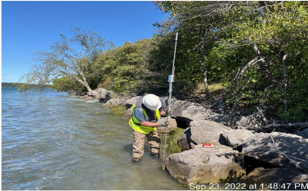
Photo 9 - Performing Dynamic Cone Penetrometer (DCP) test at Site No. 91. Note armor stone along shoreline.
