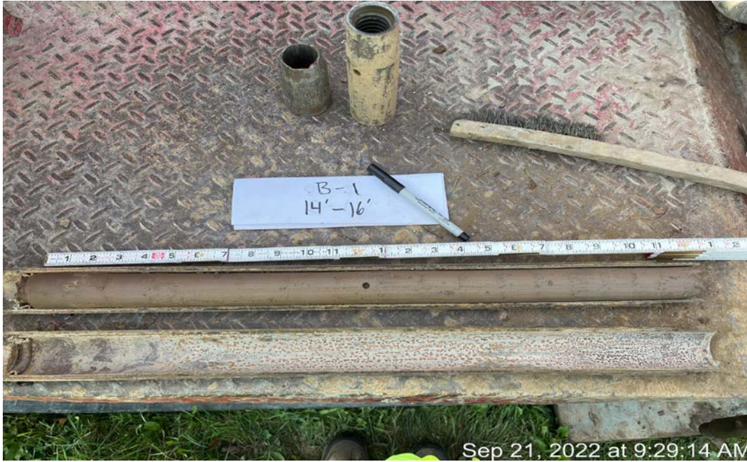
Photo 3 - Recovered split spoon sample from test boring, showing recovered core sample of Silty CLAY.
