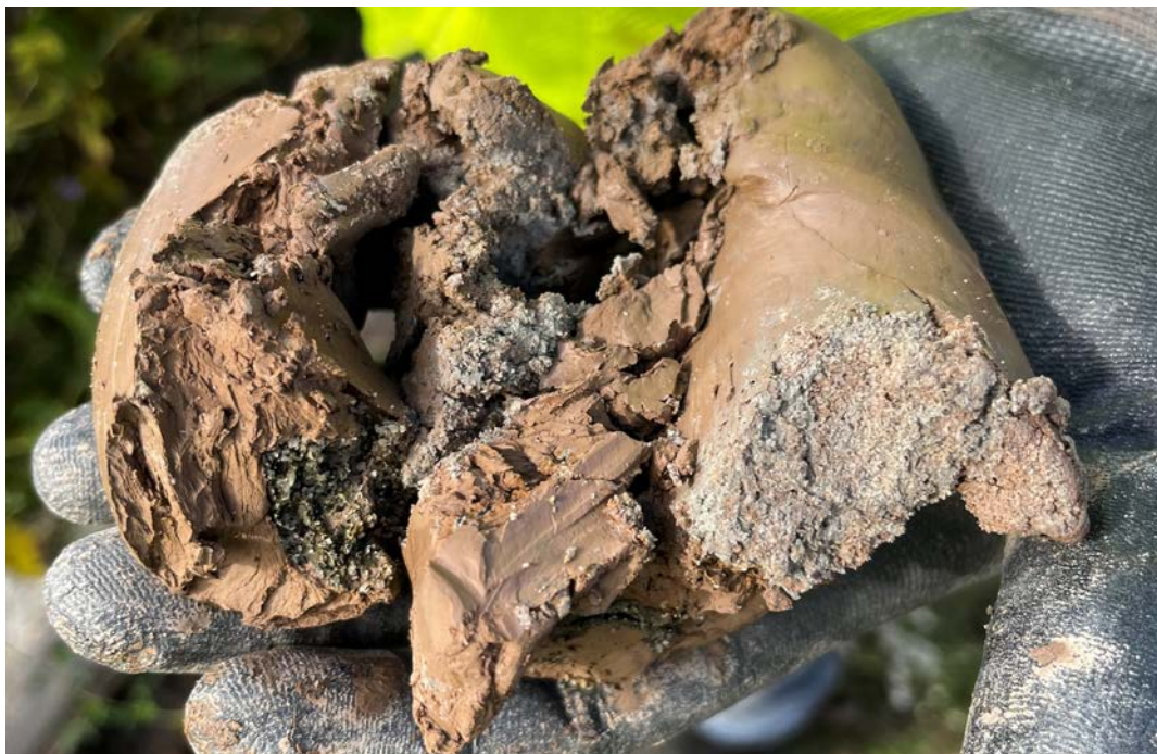
Photo 6 - Recovered soil sample from hand augering near shoreline at Site No. 85+86. Confirmation of Silty CLAY soils up to a depth of 7-feet below ground surface.
