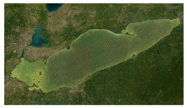
Figure 3 LEOFS-based FVCOM model domain and mesh for Lake Erie.
